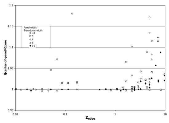
FIG. A1.1 Effect of Panel Construction on Measurement Requirements Based on the Parametric Analysis Summarized in Table X2.1
